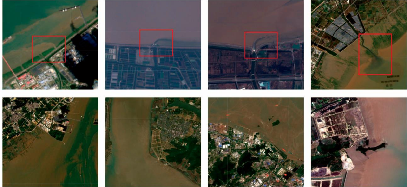
Figure 2. Supervised dataset. The first row represents samples with drainage and the second row represents samples without drainage. A red box has been added to visually highlight the location of the outfall.
